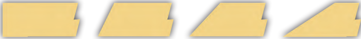
Standard bevel angles include 90°, 60°, 45°, and 30°
