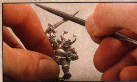
Use a needle file to remove any mould lines prior to undercoating the model.
