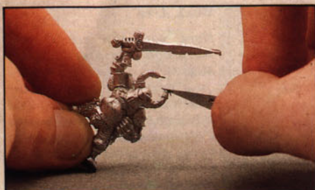
Carefully clean your model by cutting away any metal flash with a sharp knife. Always remember to cut away from your fingers.
